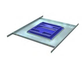
Reducing windows are used for several reasons. These include using smaller sheets of plastic on a larger aperture vacuum forming machine and also to reduce the amount of plastic in order to control the webbing which can occur on the corners of some tools.
