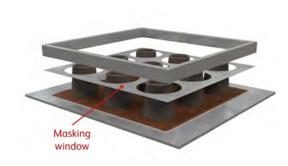
The masking windows are usually produced in sheet aluminium or steel but if need be, a simple rigid card covered in tin foil can be used for a few vacuum formings.
