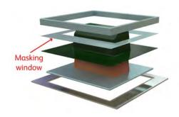
These are used to restrict the amount of heat to the sheet during the heating cycle in order to reduce the possibility of webbing caused by an excess of material.
