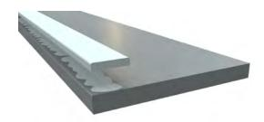
Silicone foam strip glued to aluminium or steel plate with silicone sealant. It is best to use silicone sealant to hold down the silicone foam strip to the aperture plate or bottom reducing window. We use a medium density closed cell foam sponge silicone with a Shore hardness of 5 on our smaller machines.
