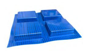
Multiple tooling can create une-qual material stretching on the sides.
